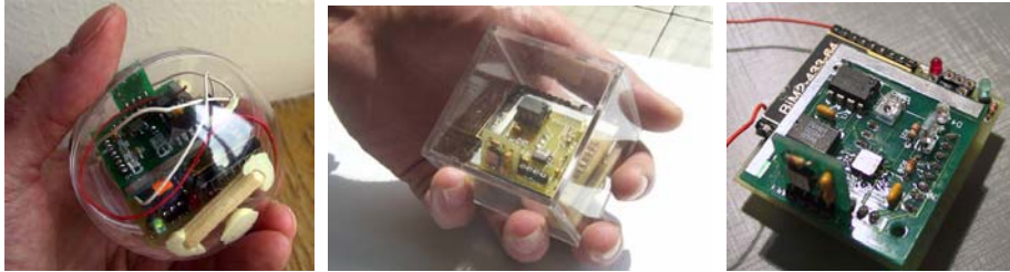
Fig. 2. In the initial design phase we explored different physical manipulation devices. The examples shown here are a sphere (left) and a cube (middle). These devices are built based on – Smart-Its - a platform for prototyping ubicomp applications.
