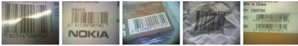
Figure 3: Successfully recognized codes : The above pictures show that our algorithm can handle reflections and shadows as well as slightly crumpled paper.
