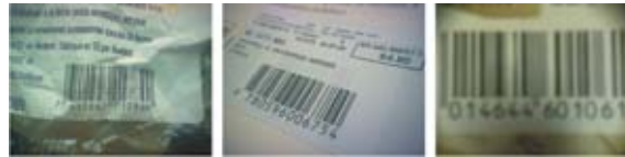
Figure 4: Unrecognized codes : The above three codes are examples of failed recognition attempts. The leftmost image shows a too crumpled bar code; the middle one is angled just too much (we only used horizontal scanline in this experiment); the rightmost image is too blurry.
