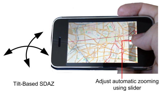
Figure 1: A prototype of a Semi-Automatic Zooming interface for map navigation. The user navigates the map with tilt and SDAZ, but can also manually adjust the zoom level with a slider (right).
