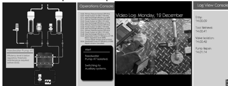
Fig. 3 Operator's Console showing alert and current status Fig. 4 Operator's console showing video log data collected by camera tracking the Ultra-Wideband beacon.
