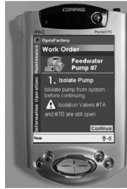
Fig. 2 Technician's Bluetooth mobile device waiting for closure confirmation from the isolation valves.
