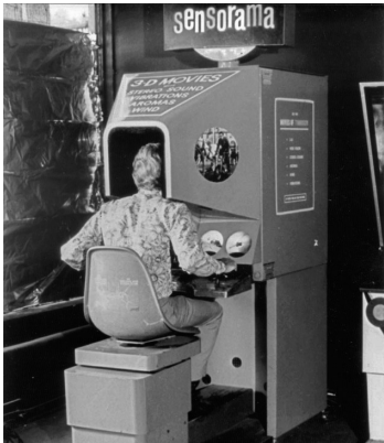
Figure 7: The Sensorama machine with sights, sounds, wind, smells and a rumbling motorcycle seat and vibrating handlebars [2].
