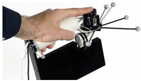
Figure 5: A prototype by Microsoft for haptic feedback in a 3D controller [5].
