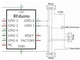
**Figure 4:** Design of the EMS control circuit.
