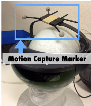
Figure 3: A motion capture marker attached to the top of HoloLens.
