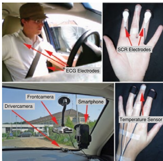
Figure 1: Study setup: Two cameras and a smartphone are placed within the car (bottom left). The driver is connected to electrodes measuring the Heart Rate (top left). Skin Conductance Response (top right) and Body Temperature (bottom right) are measured at the drivers left hand.
