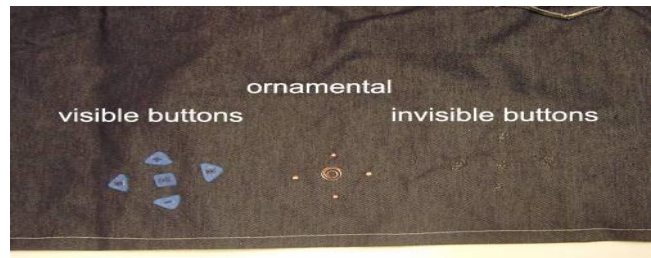
Figure 6: A close-up of the apron with the 3 different designs of the touch buttons.
