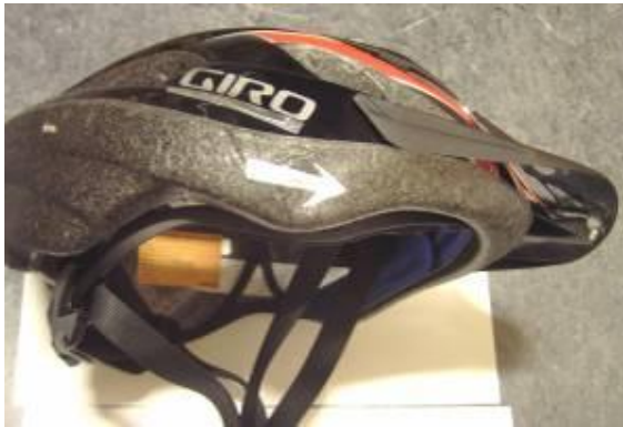
Figure 4: An off-the-shelf bicycle helmet that has been equipped with touch sensitive areas on both sides ('GIRO' logo and the arrow). A lamp in the front can give feedback.
