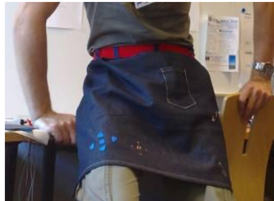
Figure 8: The apron worn by a user and adjusted such that the visible set of controls is located on the upper thigh as used in Study II.
